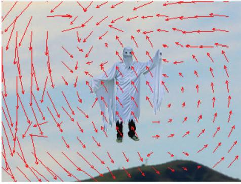
Fig. 1. This shows the detected motion paths of blocks across the image after one iteration of the affine search on the full-scale image. (see Figure 3 for the images used in this registration). The necessity of an iterative search approach is shown by the number of apparently random motion paths that are produced.
