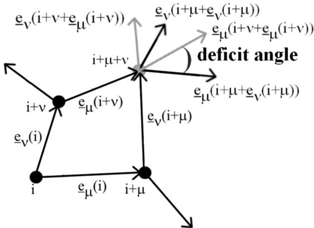
FIG. 2. A diagram showing how, when we start flattening at a point  $i$ , we obtain two different versions of the basis vectors at the diagonally opposite point  $i + \mu + \nu$ , depending on whether we respect the cell based at  $i + \mu$ , or the cell based at  $i + \nu$ . The difference between these two versions is the *deficit angle*, as shown in the diagram.
