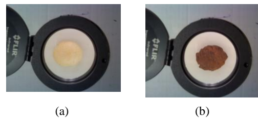
Figure 7 Image series of pastry samples taken during the cooking process: (a) a light brown pastry sample with the reference white tile background and (b) a dark brown pastry sample with unsaturated reference white tile background
