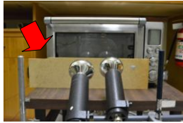
Figure 3 A wooden guard placed at the front door of the oven
