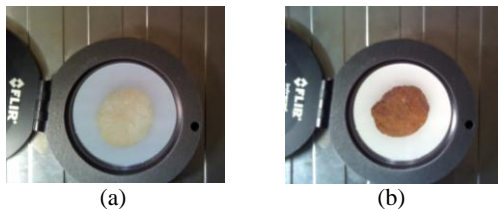
Figure 5 Image series of pastry samples with self adjustment of the camera during the cooking process: (a) a light brown pastry sample with the reference white background and (b) a dark brown pastry sample with saturated background
