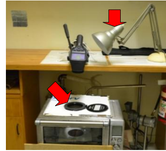
Figure 6 The light bulb above the oven and the white cardboard on the oven to overcome self adjustment issue
