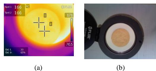
Figure 8 Pictures captured by the FLIR infrared camera: (a) an infrared image and (b) a regular colour image
